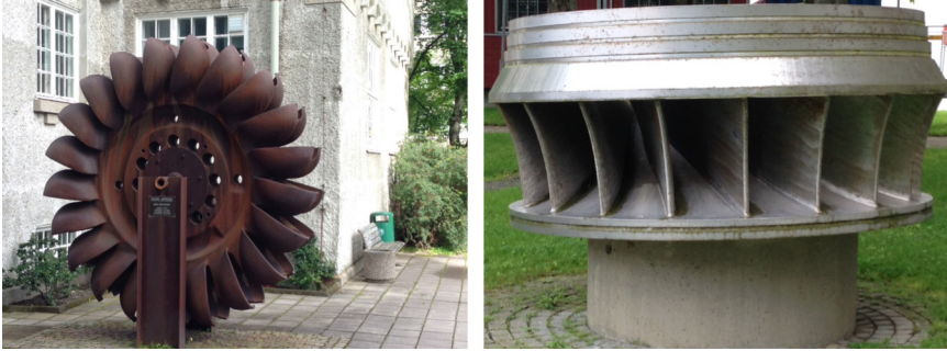
Figure 3.3 Pictures of a Pelton turbine wheel (left) and a Francis turbine wheel (right).
